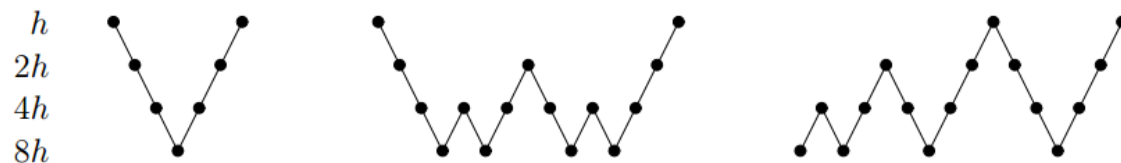
Figure 6.11: V-cycles and W-cycles and FMG use several grids several times.
